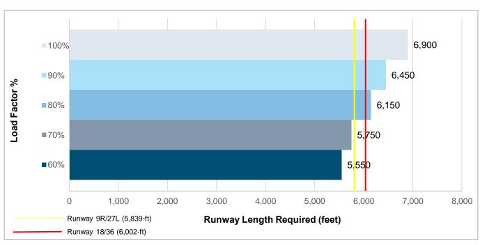
Figure 4-19 - Airbus A320 - Takeoff Distance Required - Standard Day (59°F)
