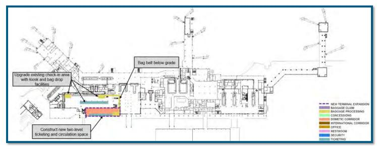
Figure 5-14 - Terminal Services Development Alternative 1: Second Floor
