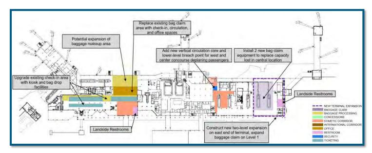
Figure 5-18 - Terminal Services Development Alternative 3: Second Floor
