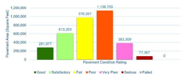
Figure 2-13 - APER's Figure 4.1.2 (b) - Latest Condition - Taxiway Pavements
